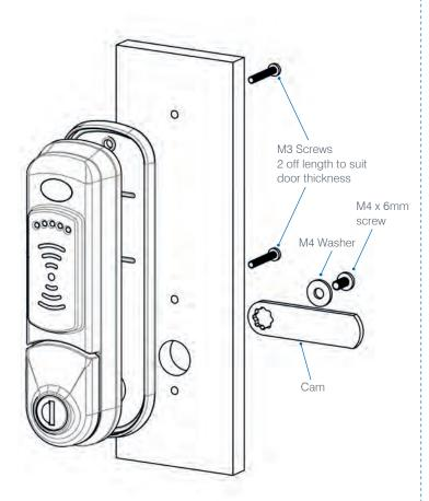
HOLES A, B & C DIAMETER 3.5 / 4.0mm HOLE D DIAMETER 16.0 / 16.5mm ALWAYS USE FIXING HOLE A USE EITHER OR BOTH OF HOLES B & C Recommended screw fixing torque 0.8Nm
